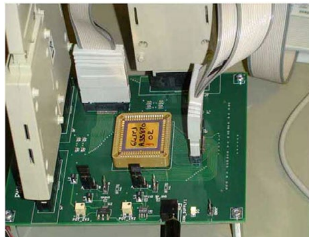
Caption: Test board and ASIC incorporating a double-memory programmable and configurable PWAG controller
